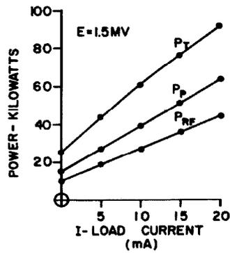
Fig. 10. Calculated load-power curves.
