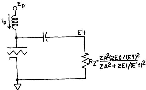
Fig. 4. Simplified oscillator circuit.
