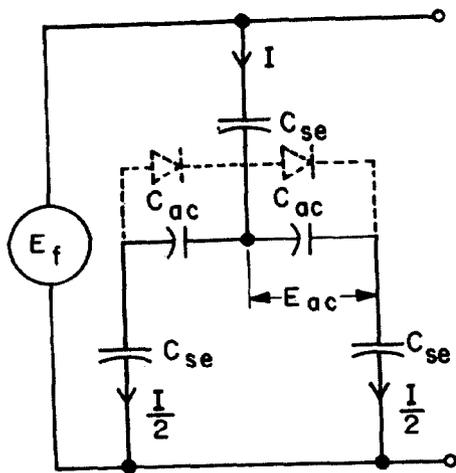
Fig. 2. Single-stage capacitive circuit.
