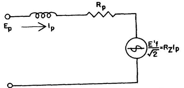
Fig. 5. Equivalent circuit of oscillator.
