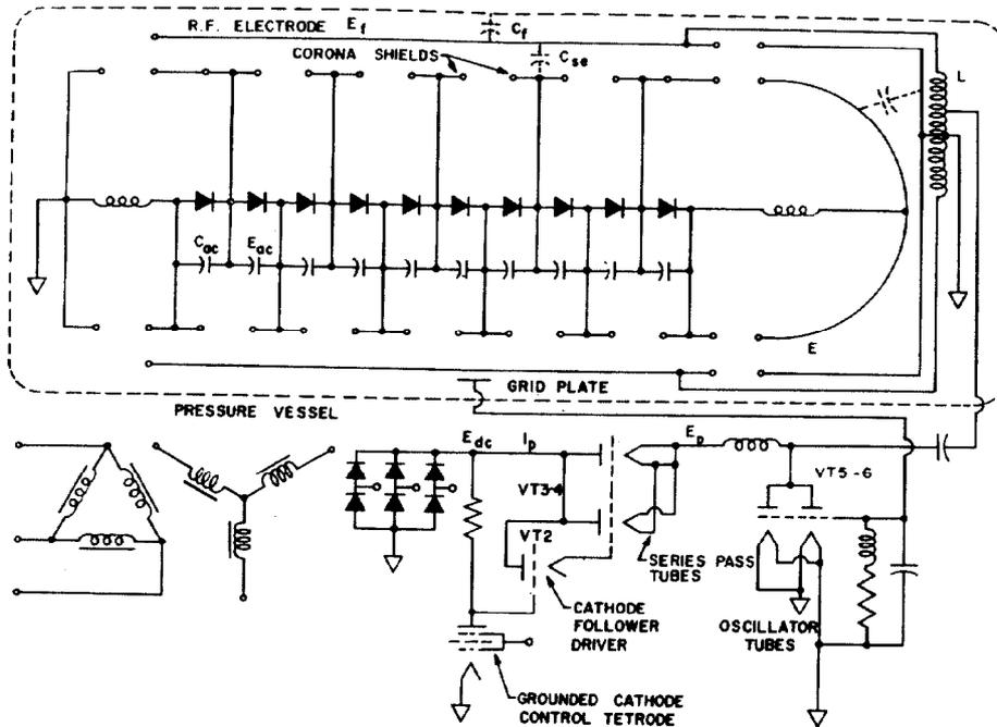
Fig. 1. High voltage generator and oscillator schematic.
