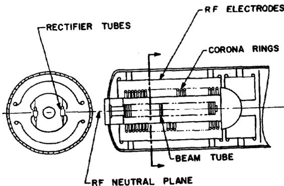
Fig. 6. Pictorial drawing of accelerator.
