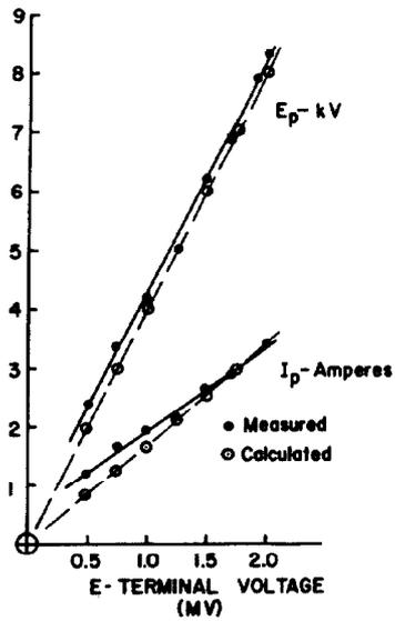
Fig. 8. Oscillator  $E_p$ - $I_p$  characteristics-no load.
