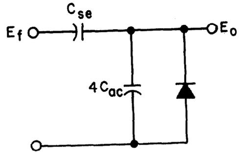
Fig. 3. Single-stage equivalent circuit.
