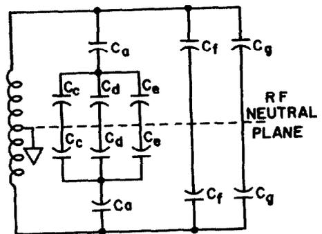
Fig. 7. Oscillator tank equivalent circuit.
